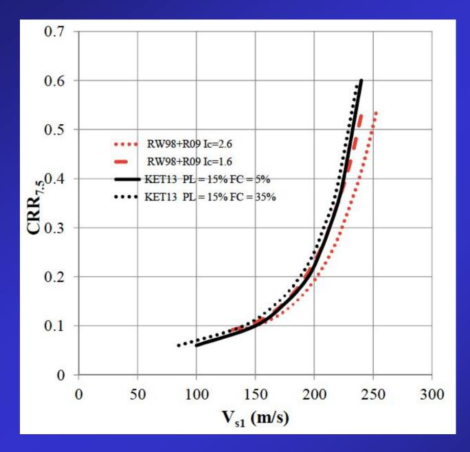
Comparison between V<sub>s1</sub>based trigger curves by *Kayen et al (2013)* and the
