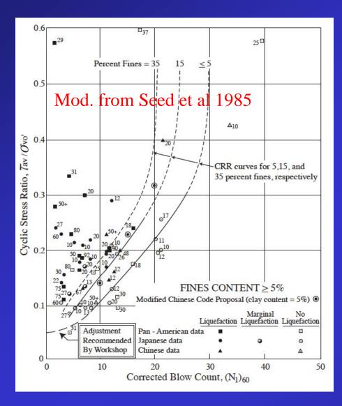
Following the 1964 earthquakes in Alaska and Niigata the "Simplified **Procedure**" was developed by Seed & Idriss (1971) for evaluating seismic demand and liquefaction resistance of sands based on case histories (liq. & non-liq. cases)
