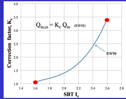
Clean sand equivalent normalized cone resistance,  $Q_{tn,cs}$  based on soil behavior type index,  $I_c$
