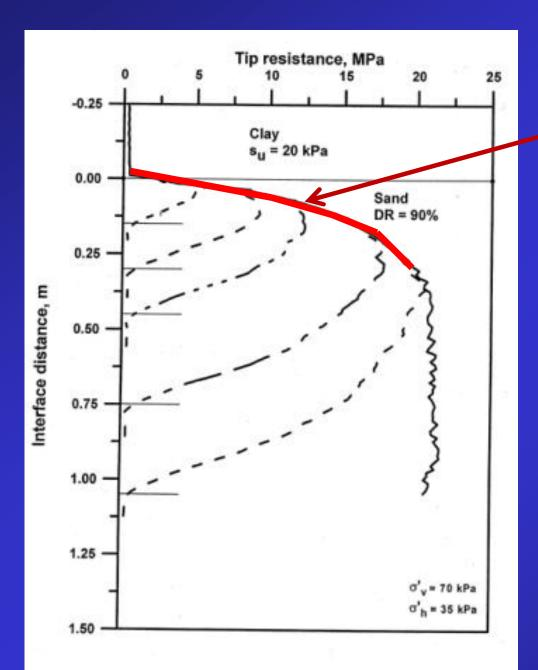
CPT data in 'transition' when cone is moving from one soil type to another when there is significant difference in soil stiffness/strength (e.g. soft clay to sand)
