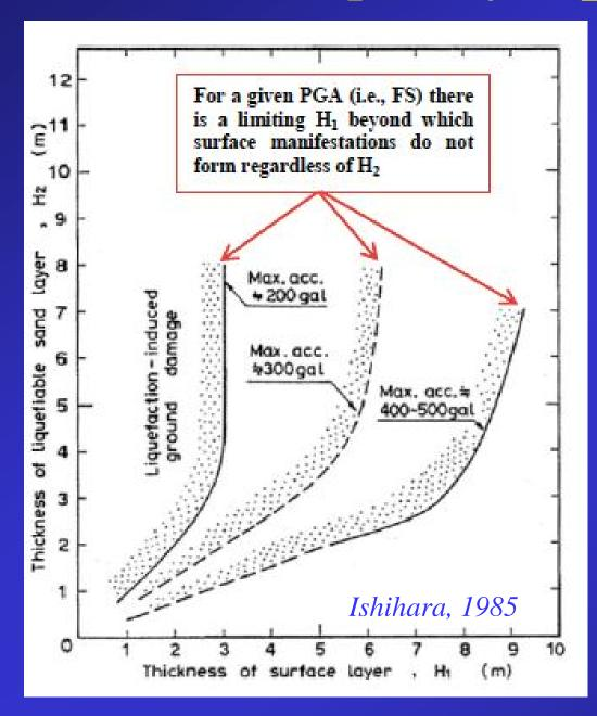
Ishihara (1985) showed that surface damage from liquefaction is influenced by thickness of liquefied layer and thickness of non-liquefied surface layer.
