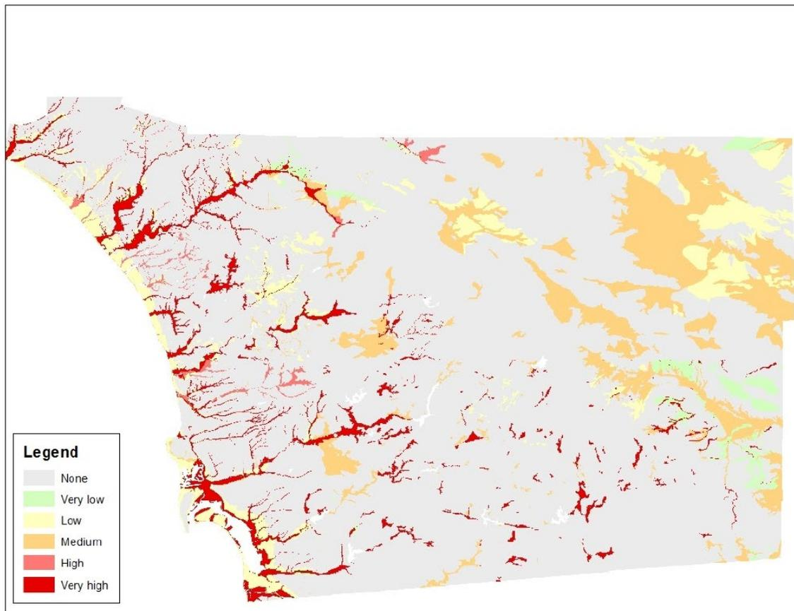
Figure 1. Liquefaction Susceptibility (LS) Map for the San Diego Earthquake Planning Scenario Report, 2018.
