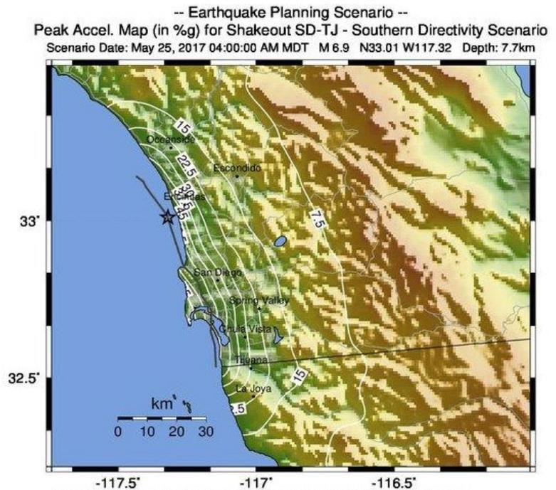
Figure 3. Earthquake Scenario Peak Ground Acceleration Map (USGS, 2017)
